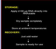
**Figure 2. Protocol for RNA storage in RNAstable.** RNA samples are applied directly into RNAstable, dried, and then stored at ambient temperatures. Sample recovery requires one-step rehydration, and the RNA is ready for use in downstream applications without the need for further purification.
